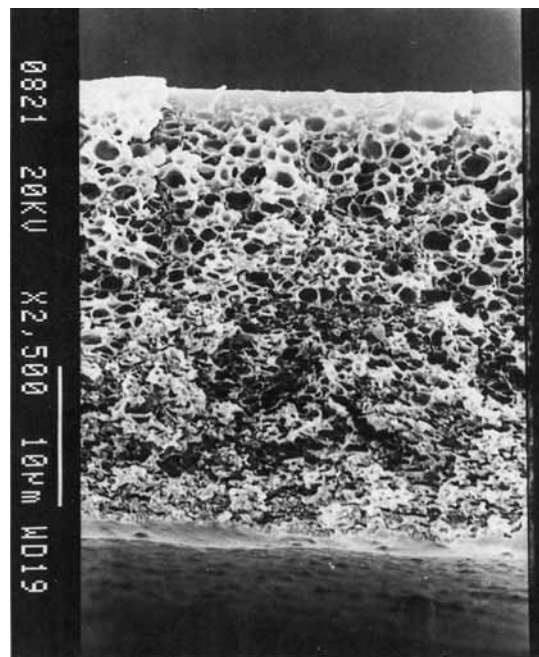
Figure 1 SEM micrographs of the cross-section of the CA membrane; 20 wt %, 300\ \mu\text{m} .
